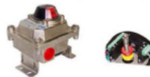
The AS-i flameproof valve monitor is a rotary valve position indication device. Armed with AChem I/O+sensor Module, the device can sensor the valve position (on/off), communicate with ASI master and output voltage (24VDC-1.5W) to operate the solenoid valves or relays based on the command from Master and PC.
